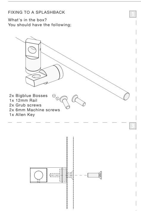
Using the M6 Screw provided, hold the boss in place [making sure the branding is in the upright position] and affix from the rear of the splashback making sure the screw head is flush below the rear surface. If the splashback does not already have holes, mark and centre punch two suitably spaced hole positions on the front of the panel ensurening they are level and at a practical height. Pilot drill using a 3mm drill-bit, then carefully enlarge the holes using a 7mm drill bit.
