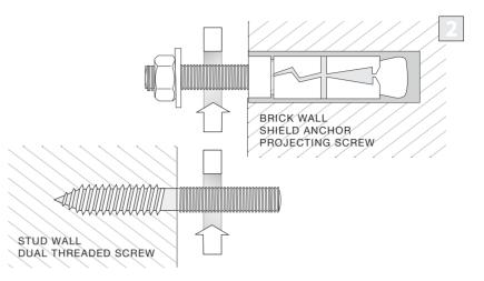
You will need the appropriate fixing, depending whether you are fixing to a stud wall or a brick wall. We recommend an M6 shield anchor projecting screw for a brick wall and an M6 dual threaded screw for a stud wall or when fixing into wood. Both are available separately from your local DIY store.
