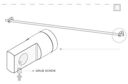
Slide the bar through the bosses making sure that there is an even amount of bar either side. Affix the bar with the grub screws provided, making sure they are tightly secured.
