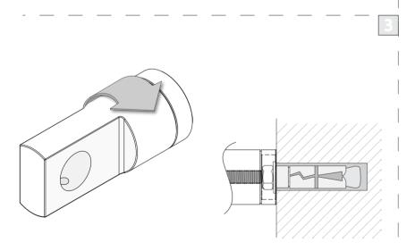
Carefully screw the boss onto you chosen fixing point ensuring that the boss is secure and the branding is positioned in the upright position. Be careful not to over tighten the boss.
