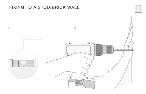
Mark two suitably spaced holes onto the surface you wish to drill, making sure they are level. Drill holes appropriate to the fixings used [see below].
