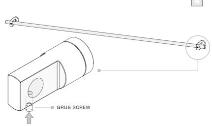
Slide the bar through the bosses, making sure that there is an even amount of bar either side. Affix the bar with the grub screws provided, making sure they are tightly secured.
